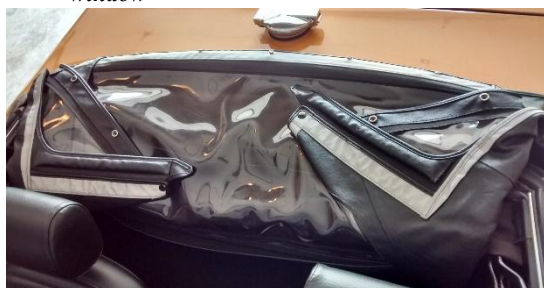
3. Fold side windows on top without folding side windows, tuck top down behind seats, add cover.
