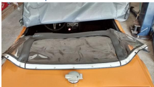
2. Fold top forward without folding back window
