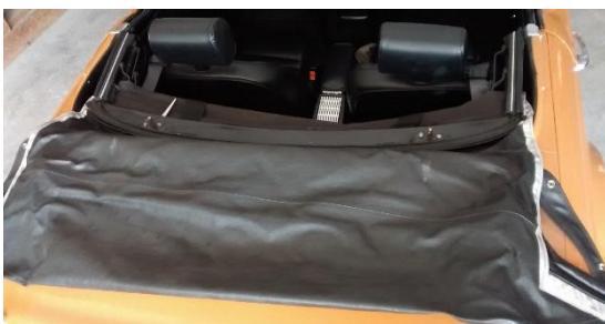
*Unsnap the top from the rear bow and beneath each side window. Spread over boot lid.*
