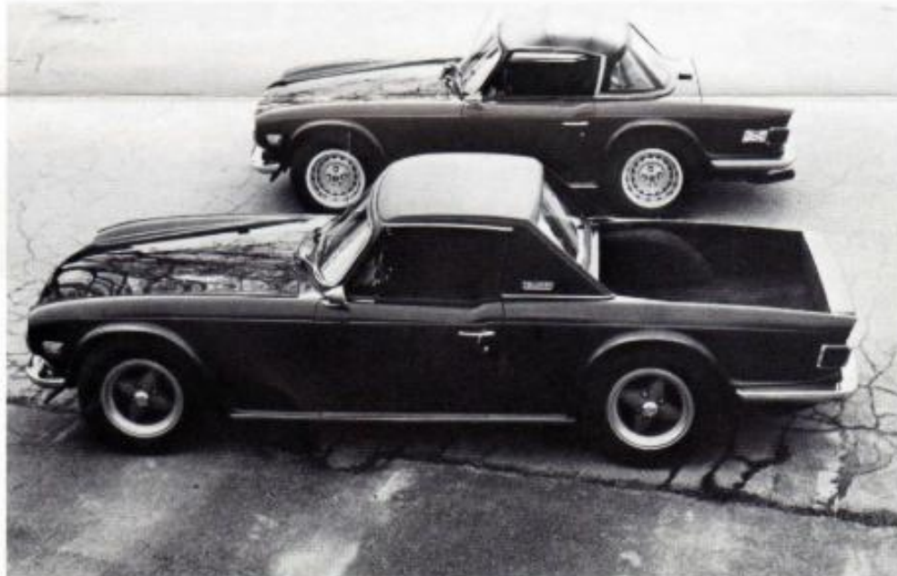
This photo shows how Roger Hurst's special TR6 pick-up is lengthened by 12in. mostly between door and wheel, to form an extremely neat and attractive design. (Photo: Dave Gilmore)
