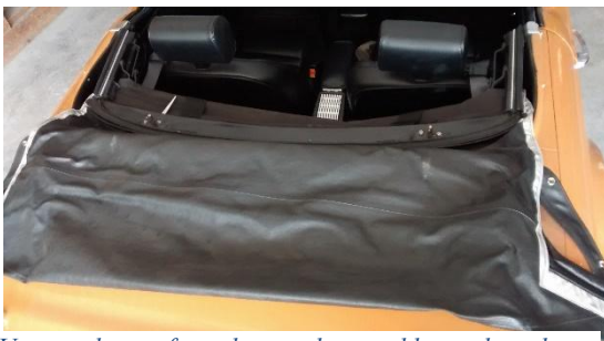
Unsnap the top from the rear bow and beneath each side window. Spread over boot lid.
