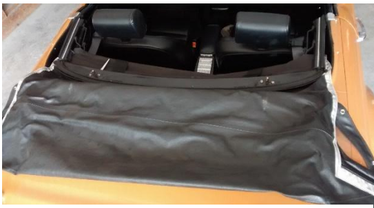
Unsnap the top from the rear bow and beneath each side window. Spread over boot lid.
