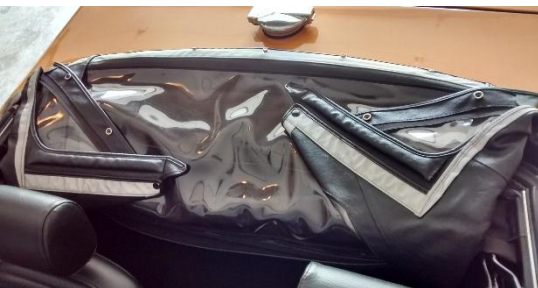
3. Fold side windows on top without folding side windows, tuck top down behind seats, add cover.
